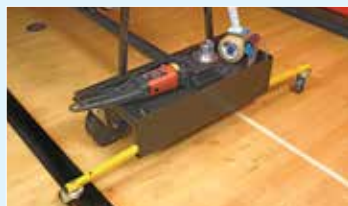
Storage trays with safety leg extenders
